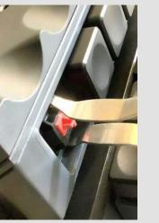
Position the secondary switch housings in the lowest position.
